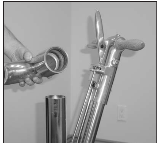
40. Clean out dust accumulation between the seals.
