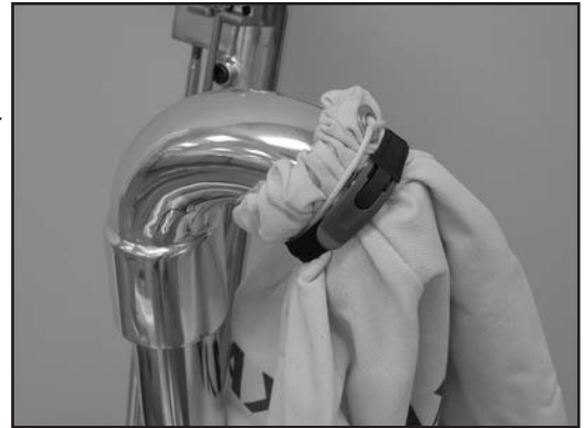
27. Secure dust bag on elbow.
