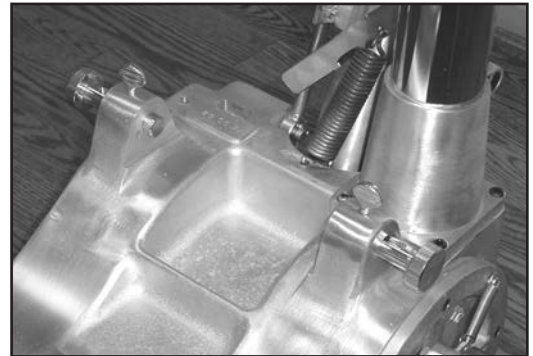
5. Make sure pins are pulled out before installing the motor.
