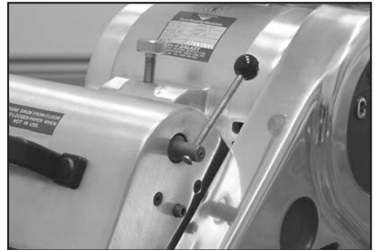
21. Disengage tension belt mechanism.
