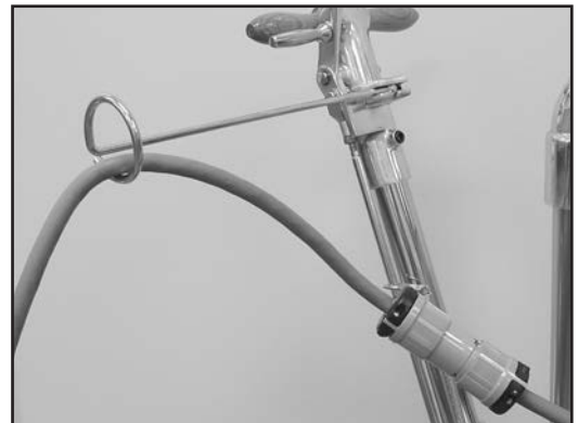
28. Keep power cord out of the path of sander.
