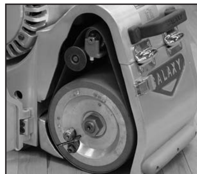
24. Set sanding belt on proper track.
