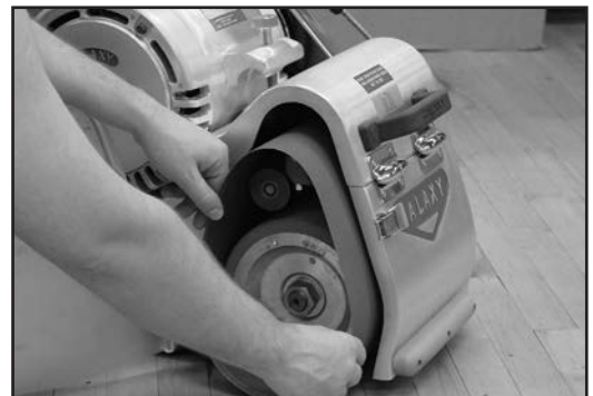
23. Slide belt into position.
