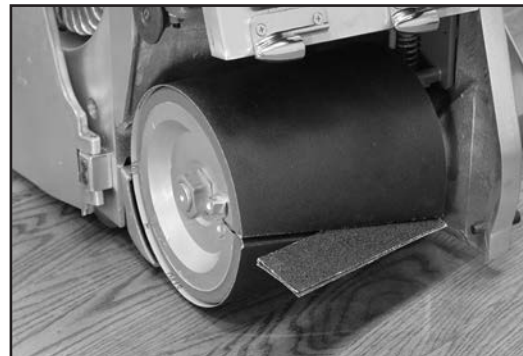
18. Insert required wedges.
