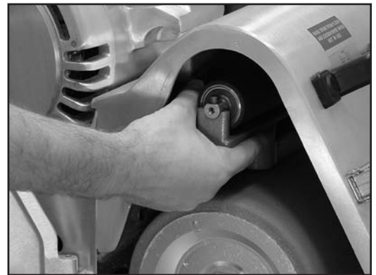
34. Remove roller mechanism.
