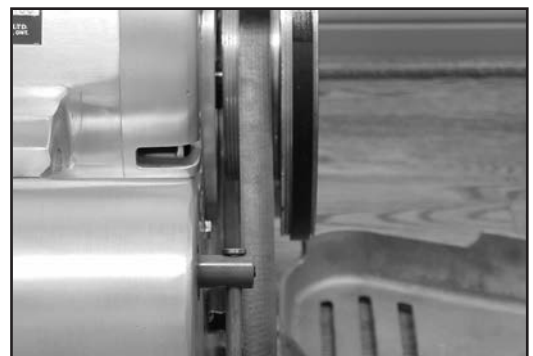
7. Line up drive belts as shown.
