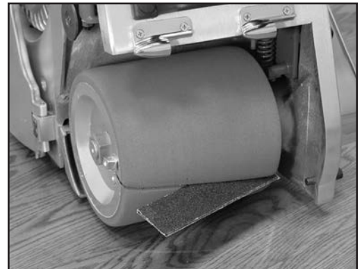
16. Remove balancing wedges.
