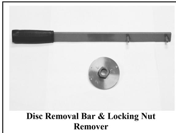
**Disc Removal Bar & Locking Nut
